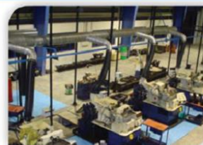
Centralized mist & Smoke extraction for Neat oil/Water soluble coolant
