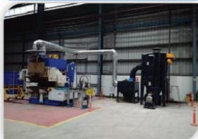
Dry Dust Collection for robotic Welding/Grinding/Plasma/Laser Cutting Operation with spark arrestor
