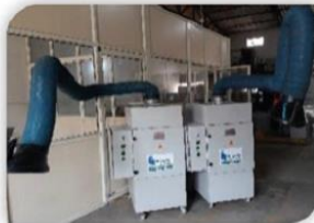
Portable Fume extractor to Extract of fume at source
