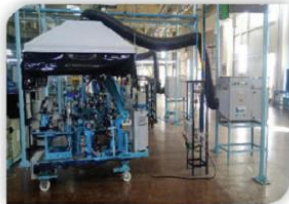
Fume Extraction for manual/robotic welding station
