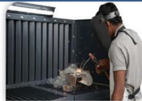
Dry Dust Collection for robotic Welding/Grinding/Plasma/Laser Cutting Operation with spark arrestor
