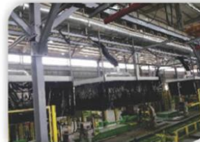
Centralized ducting system for welding fume extraction
