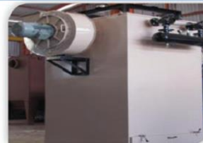
Dry Dust Collection for robotic Welding/Grinding/Plasma/Laser Cutting Operation with spark arrestor
